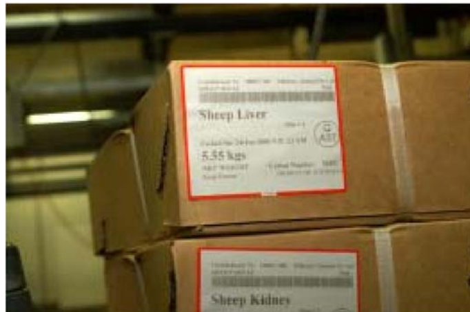
The printed carton labels comply with the GS1 Standards and the guidelines for numbering and bar coding meat products.
