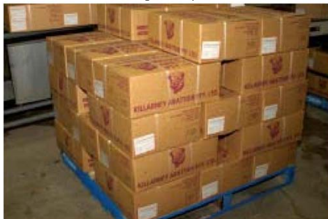
Carton product is palletted ready for shipment. The cartons and pallets are controlled through the inventory system that provide the traceability linkages from boning room to distribution.
